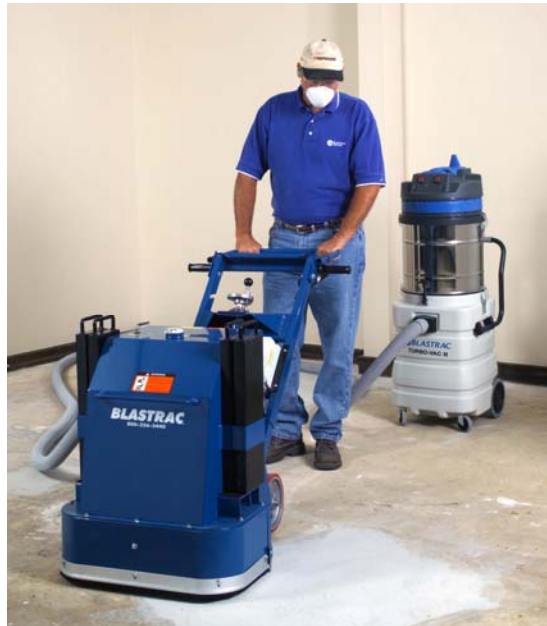
Figure 7 – Connection to dust collector
